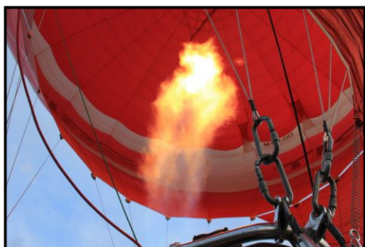
Figure 17: Burners heat up the air inside a hot air balloon.
