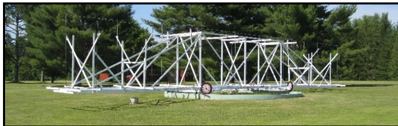
Figure 9: Full-scale replica of Karl Jansky's radio telescope at the US National Radio Astronomy Observatory.
