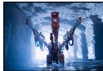
Figure 17: Drills are used in underground and surface mines to prepare the rock face for blasting.
